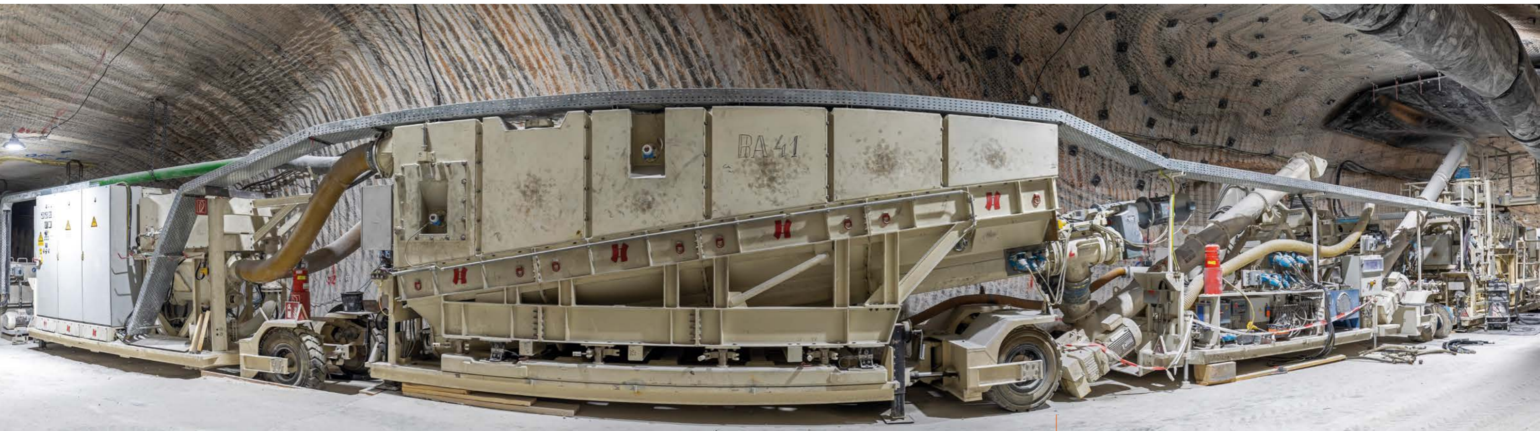
Asse mine: Semi-mobile building material facility on the 750 m level
